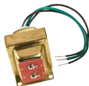
4381 Transformer W. 2.75", H. 2.50", L. 2" Optional: Necessary only when doorbell transformer unavailable for installation. 16V Output
